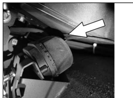
Hose connection at the vacuum pressure socket of the side brush lowering system
