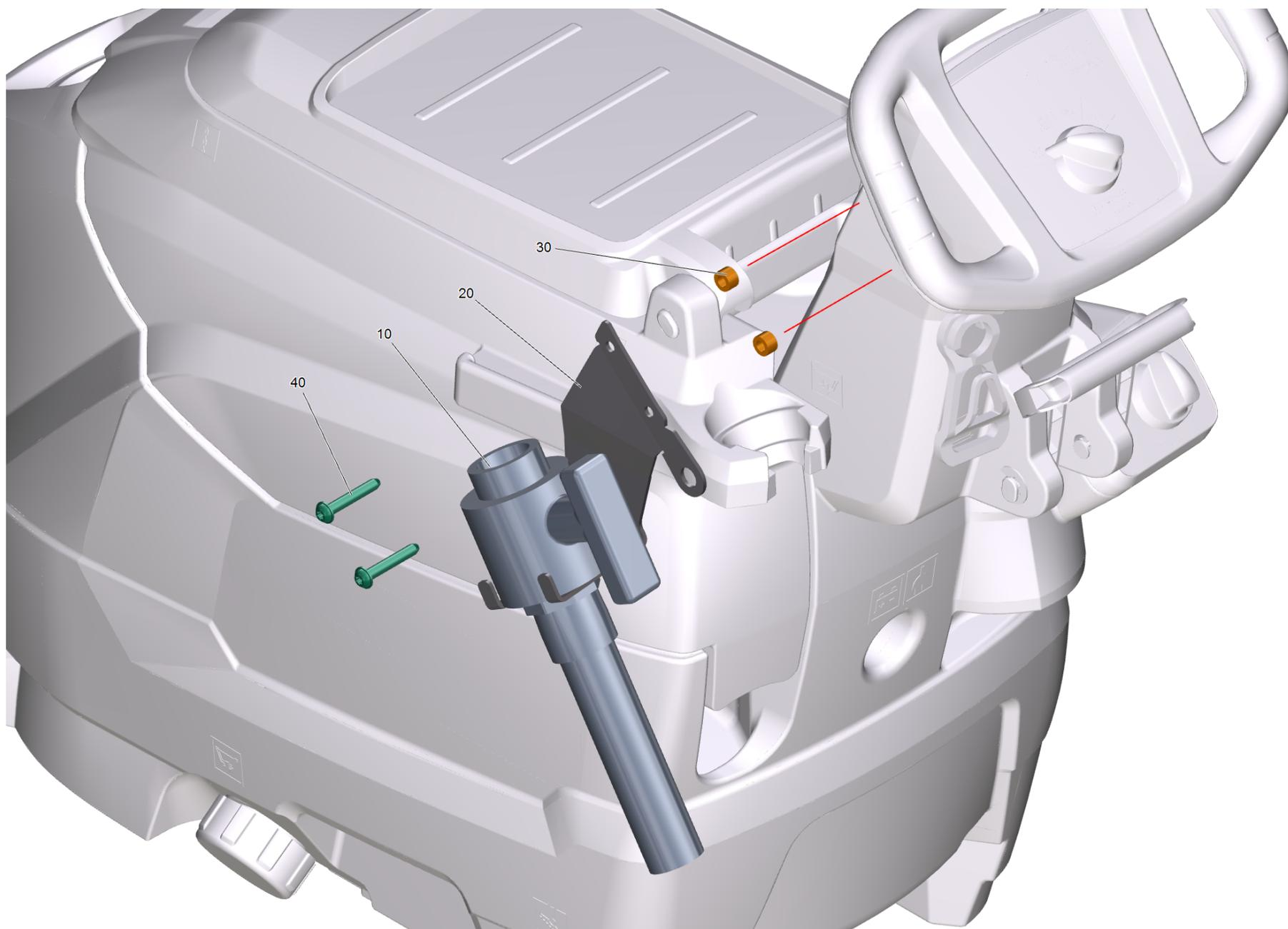
9510 ABS Ablassschlauch Kugelhahn BD 43 (2.643-977.0)
